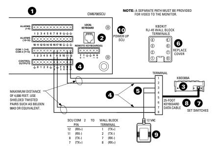
Figure 6. RS-422 Interface Connections (CM6700)
